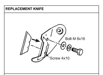
When the cutting knife is dull replace it as soon as possible.
